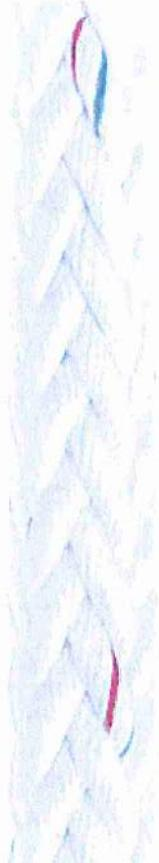
HTP-12 is a 12-strand construction that provides optimum performance in static bending situations by allowing even distribution of loads across the bend, making HTP-12 ideal for use where small D/d ratios are common. Made with high-tenacity polyester fiber to provide good flex-fatigue resistance and shock absorption, HTP-12 is available with Samson's proprietary Pro-Gard Marine Finish for enhanced performance.
